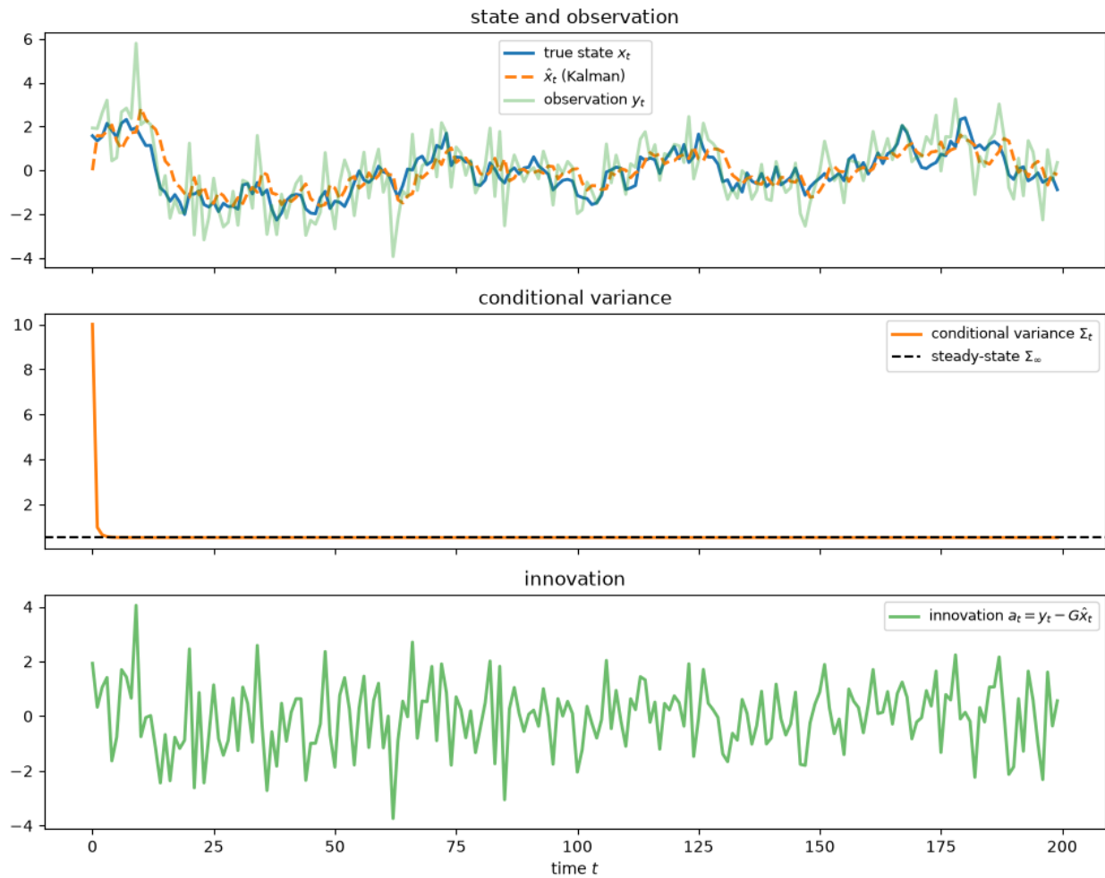
Fig. 49.1: Scalar Kalman filtering
